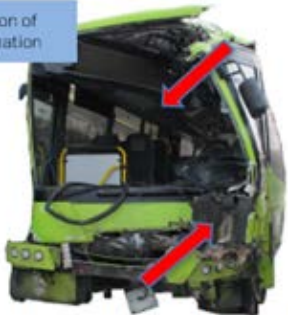
Figure 2: Damage to the front of the eastbound bus. Photo: AIBN
