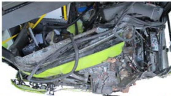
Figure 3: Deformations of the driver's cab in the eastbound bus, seen from above. Photo: AIBN
