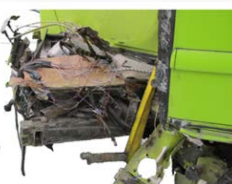
Figure 5: Cross-beam severed on the left-hand side, seen from the side. Photo: AIBN
