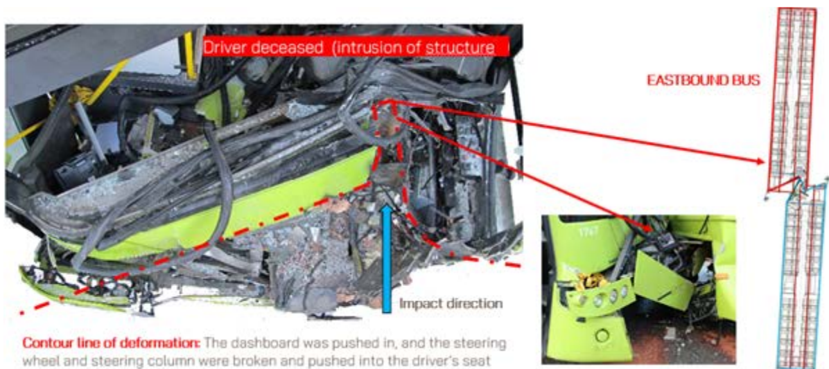
Figure 1.8: Severe intrusion after the crash [1]
