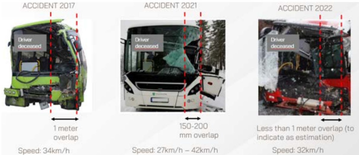
Figure 1.7: Crash overlap in the three different accidents.
