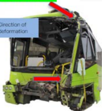
Figure 4: Damage to the front of the westbound bus. Photo: AIBN
