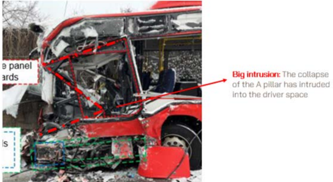
Figure 1.14: Structural status after the crash [3]
