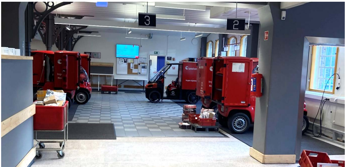
Photo 3.2: Inside one of Posten's urban depots. That the vehicles are electric and small allows them to be loaded indoors. Photo: Howard Weir
