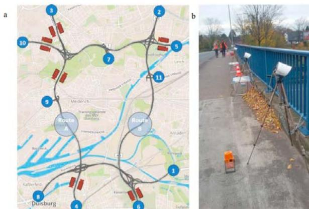
Figure 1. (a) Study network with the positions of the ANPR cameras, (b) ANPR cameras on one of the measurement positions
