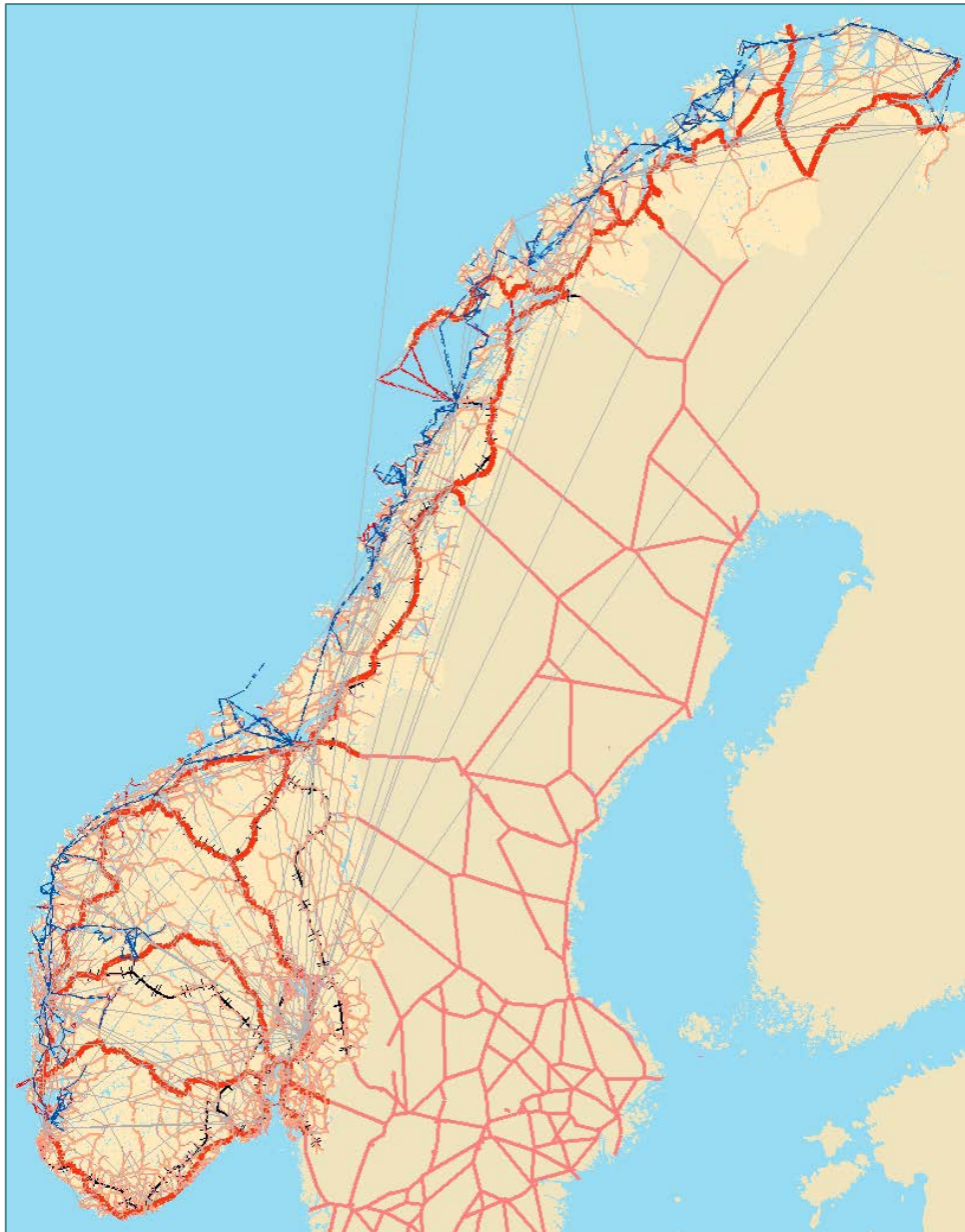
Figure E.1: NTM5 model network. Roads marked in red, railroads in black, sea routes in blue, air routes in gray. Certain Swedish roads are included, as they sometimes offer faster routes on Norwegian origin-destination pairs.
