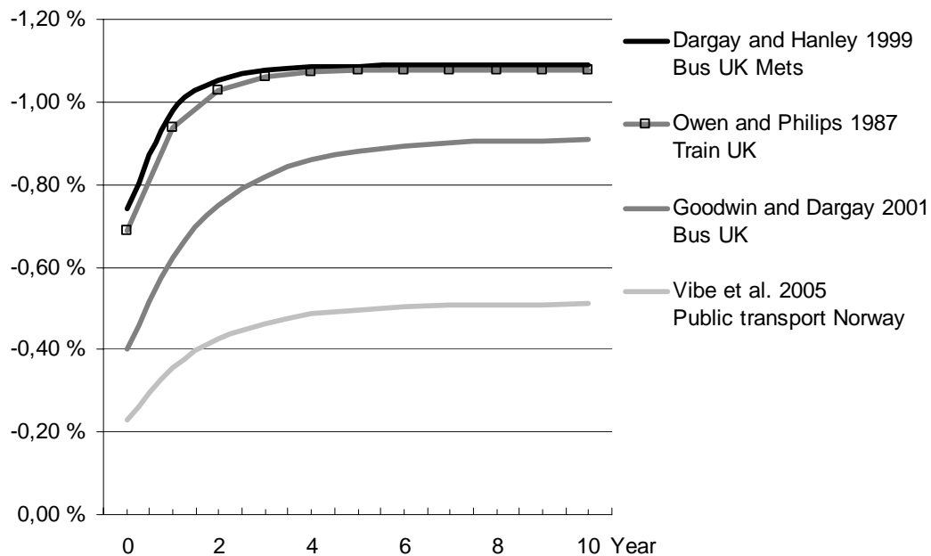
Figure 3: Dynamics of passengers' adjustments to 1 percent fare increases in year 0. Calculations based on reported coefficients in a selection of studies.
