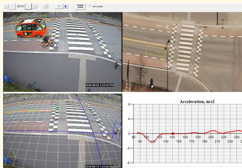
Figure 8 – An example of the analysis conducted in T-Analyst (here, the shuttle stopped hard to give way to a cyclist – video 3 )
