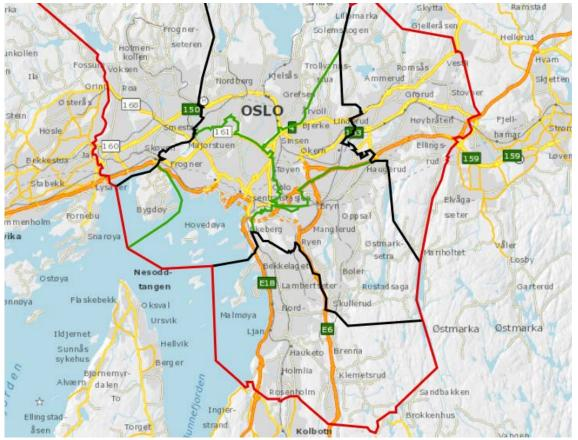
Figure 2.32: Existing and new toll-lines in Oslo (Black lines – placing of existing toll-stations, outer red lines – new city border toll-stations, green lines - new inner city toll-stations). Source: Norwegian Public Roads Administration
