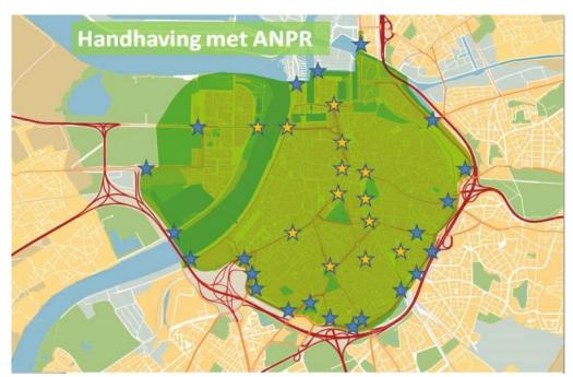
Figure 2.18: Location of ANPR- cameras in Antwerp (blue stars- cameras operating January 2017, yellow starsplanned new cameras). Source: Gazet van Antwerpen 2017
