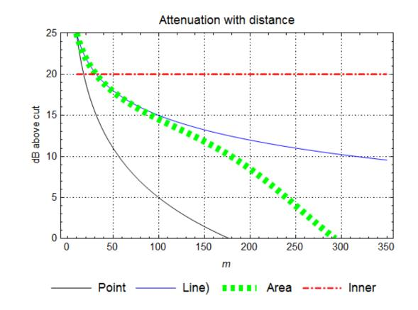
Attenuation with distance. Emitted noise 70dBA, cut off 45dBA.
