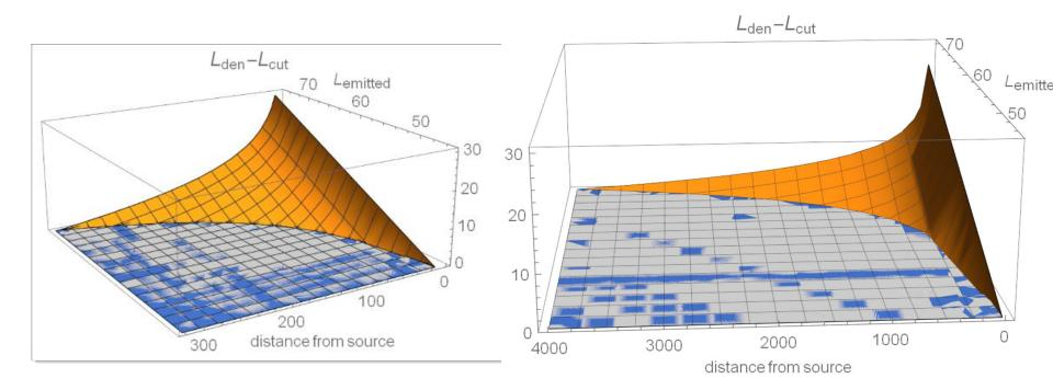
Noise exposure as a function of emitted noise and distance. Left : point source, right : line source.
