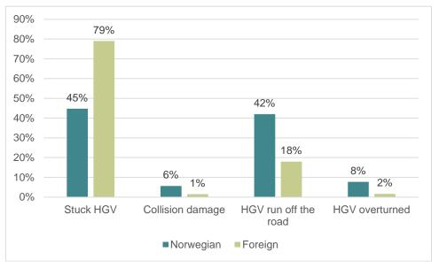
Figure 4.3 Cause of damage for foreign (N=747) and Norwegian (N=2663) HGVs that were given towing assistance and registered in the "FOU-Bilberging" project from January 1st 2013 to November 2015. Source: Falck Redning AS.
