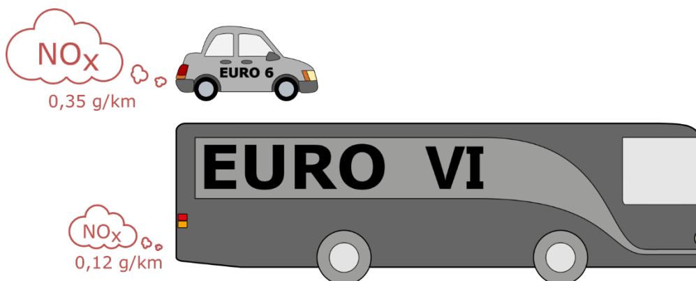
Figure S1: New heavy vehicles with Euro VI approved diesel engines have very low emission of all types of local emissions. NO x emission from new passenger cars with Euro 6 diesel engines under demanding city-driving conditions is still a challenge for urban air quality. The emissions shown are typical for demanding city-driving for passenger cars and city-buses, respectively.
